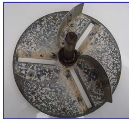
Cutter has been neglected and shows severe mineral deposit buildup. Regular cleaning and maintenance would have prevented this.
